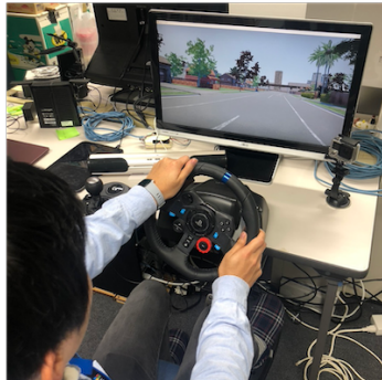
Figure 3: The Wizard-of-Oz setup. [Top] The overhead view of the room with the location of participant, researcher and assistant. The researcher sees a mirror of the participant's monitor. Every time the driver comes near a decision point, the researcher plays the recorded instructions and conversations. [Bottom] A participant using the setup. In front are: 1 monitor for driving simulator, 1 GoPro camera for capturing utterances while thinking aloud, 1 steering wheel set, and 1 speaker.
